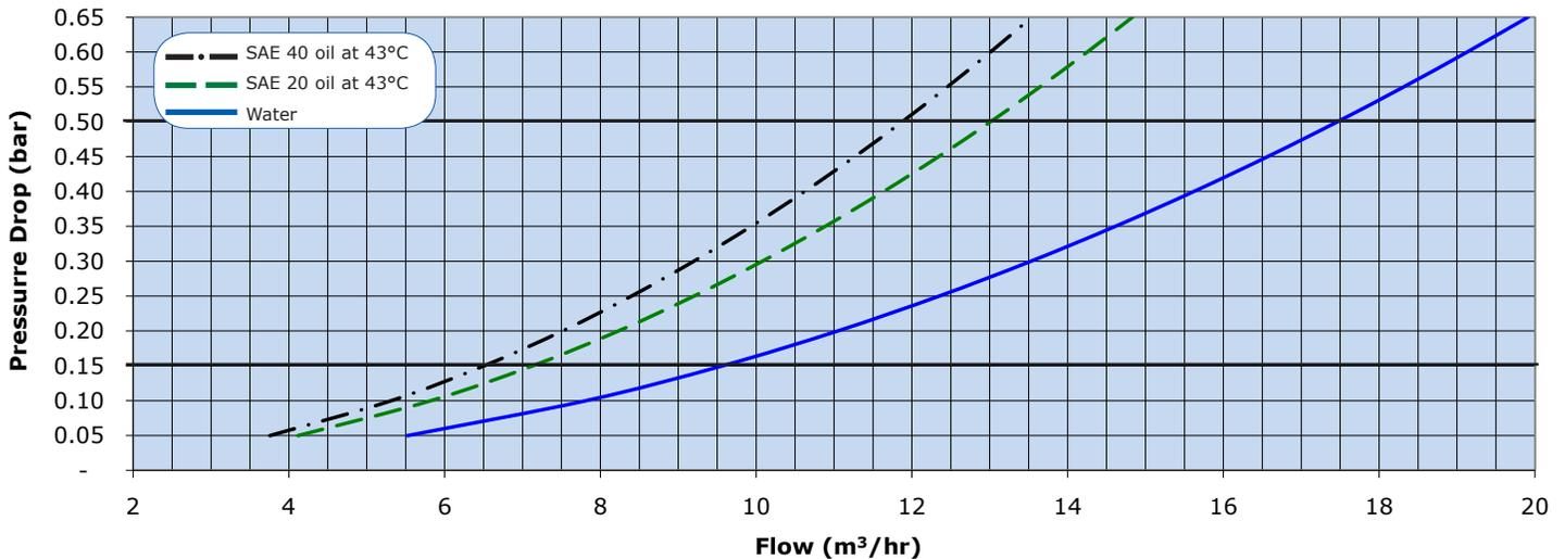
AMOT thermostatic valves are designed to produce minimal pressure drop. The normal recommendation in sizing the valves is to select a pressure drop between 0.14 to 0.5 bar (2 to 7 psi).
